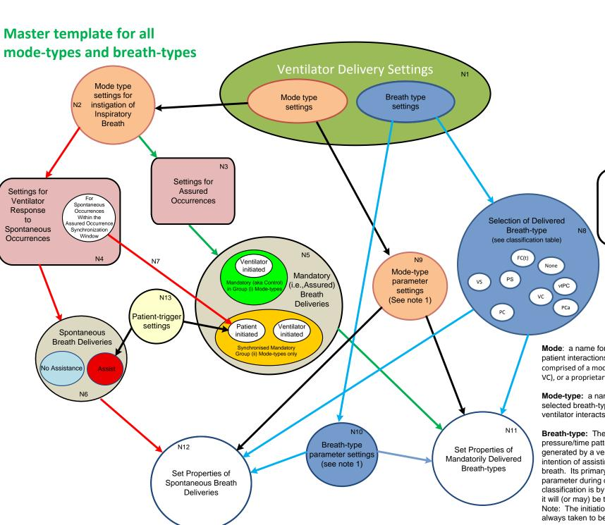
Note1: The breath and mode-type parameters settings are settings which may be changed by the operator or may be adjusted continuously or incrementally, in accordance with the selected algorithm by using feedback from measured parameters
