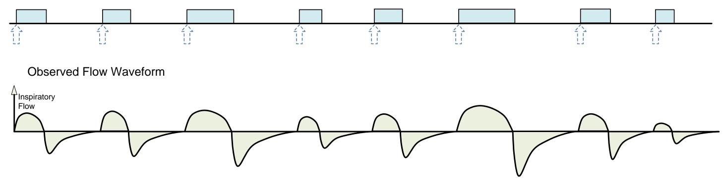
In this illustration a pressure support breath-type has been selected. This provides support by maintaining an elevated pressure during the inspiratory phase which is terminated if the patient makes an expiratory effort. The top delivery pattern illustrates the operator's perspective when setting the ventilator. The waveform below it illustrates a typical resultant respiratory flow pattern.
