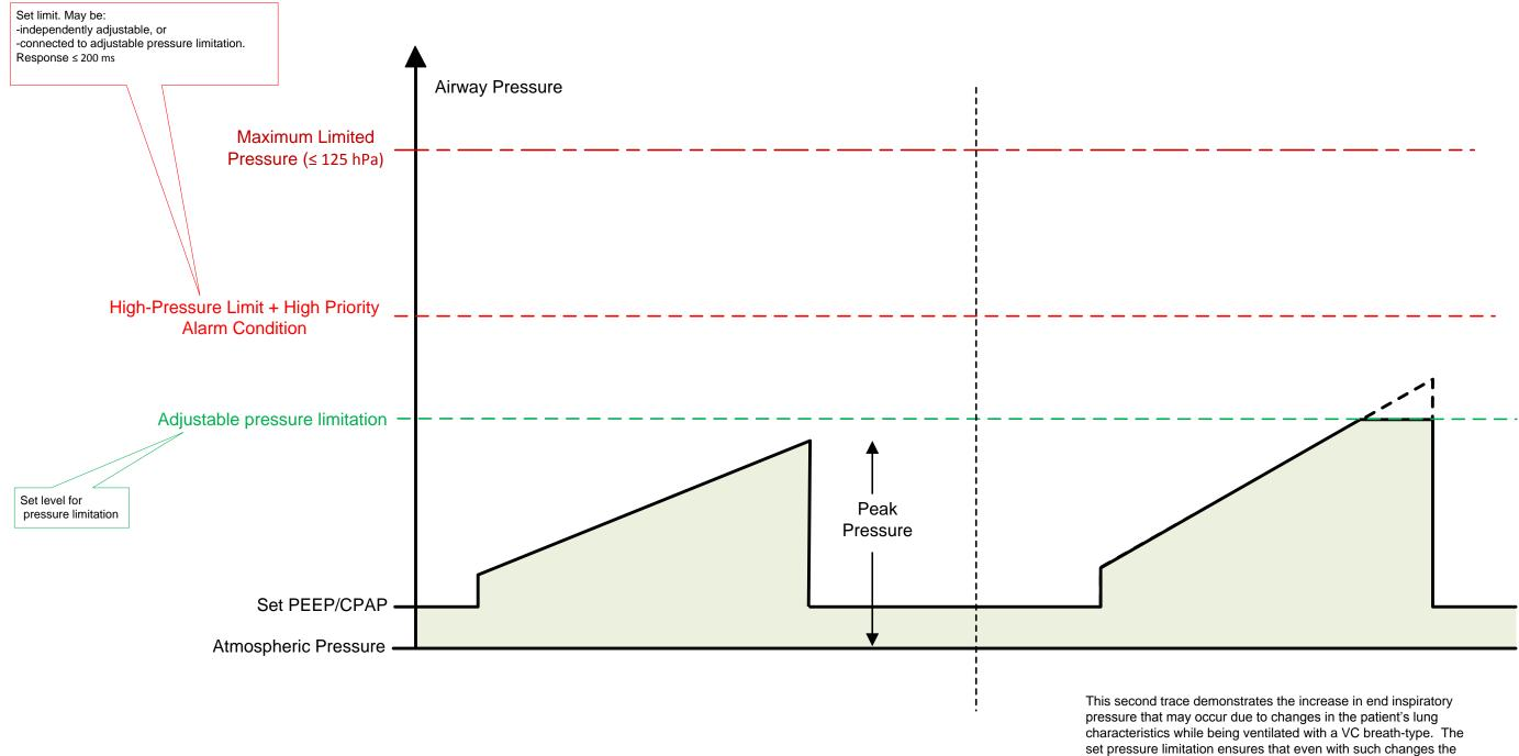
lung is protected from excessive pressure without creating a nuisance by generating alarms unless the consequent loss of delivered volume becomes excessive.
