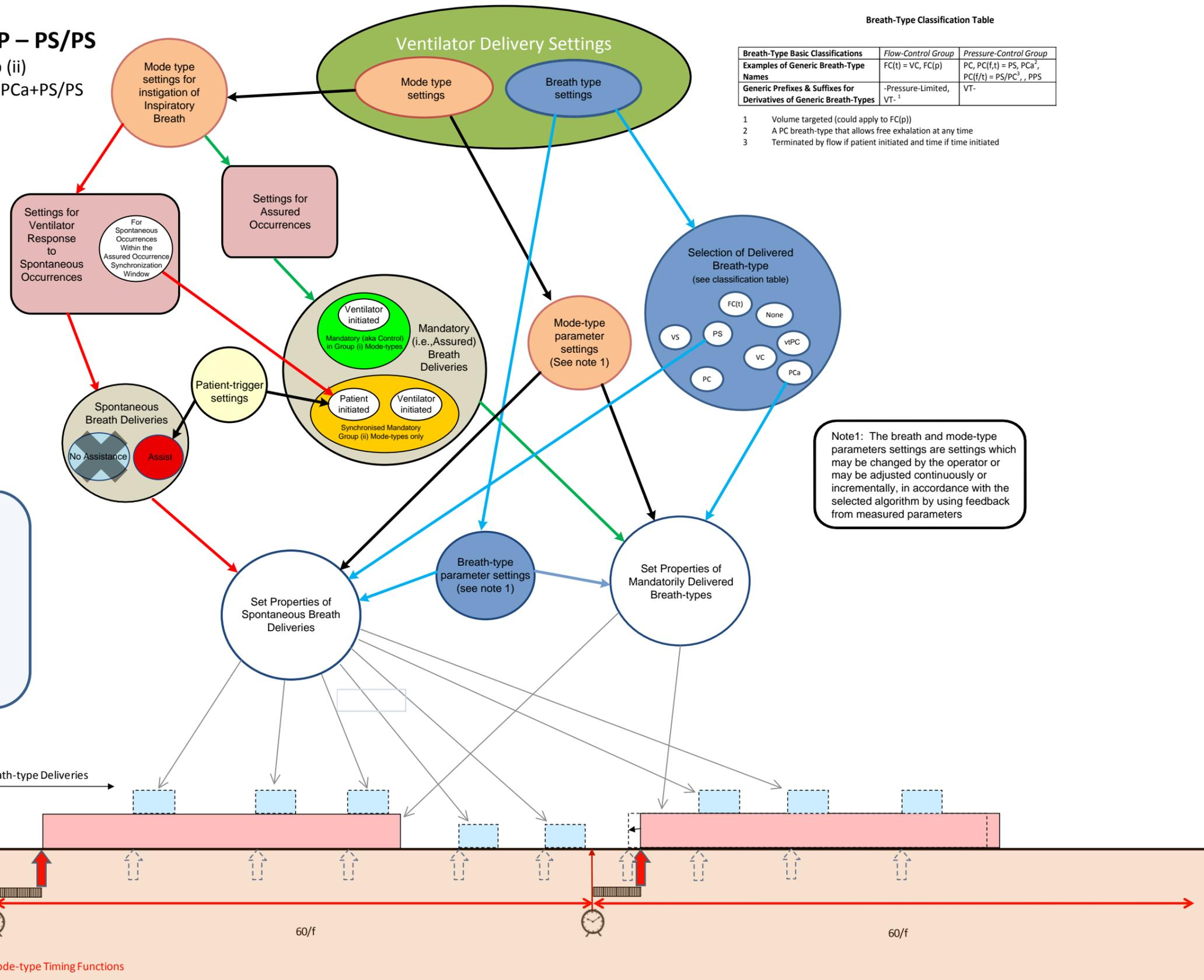
Diagrammatic representation of operator's perspective when setting a ventilator to provide a Bi Level CPAP mode-type, which uses a PCa breath-type for the Mandatory deliveries and a PS breath-type for the Assist deliveries at both high and low pressure levels.
