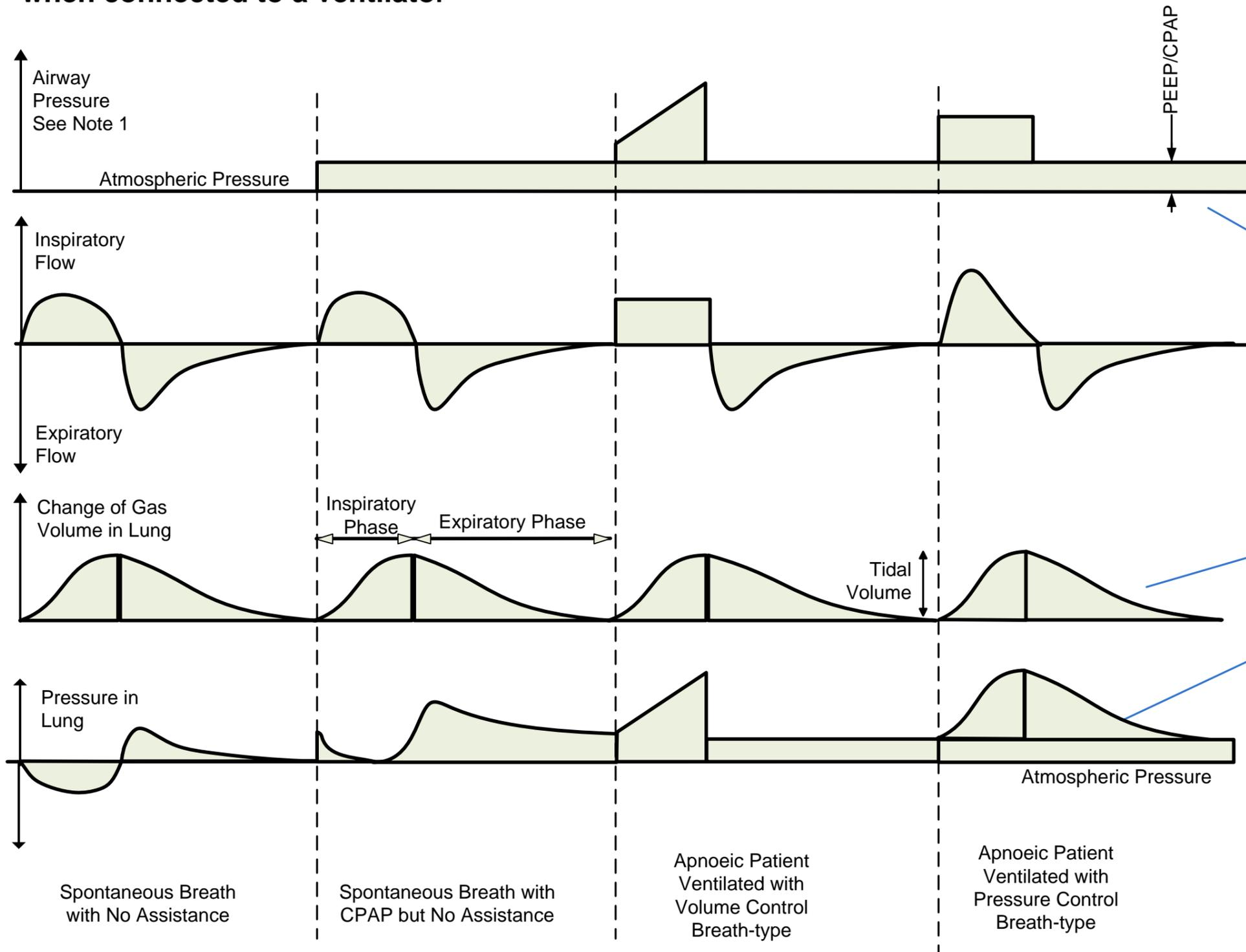
When a patient is connected to a ventilator the inspiratory volume is known as the **delivered volume** and the exhaled volume is used to determine the **tidal volume** (as that is the volume that has gone in and out).
