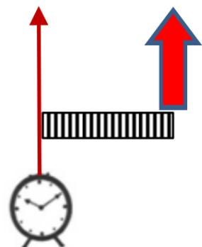
This composite symbol represents the function of a synchronization window. After instigation by an assured occurrence it provides time for the exhalation of any previously inhaled breath but responds immediately to a spontaneous occurrence by initiating the already assured breath-type delivery.
