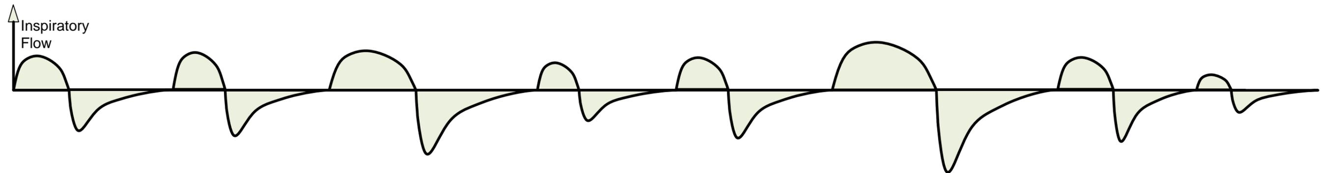
In this illustration a pressure support breath-type has been selected. This provides support by maintaining an elevated pressure during the inspiratory phase which is terminated if the patient makes an expiratory effort. The top delivery pattern illustrates the operator's perspective when setting the ventilator. The waveform below it illustrates a typical resultant respiratory flow pattern.
