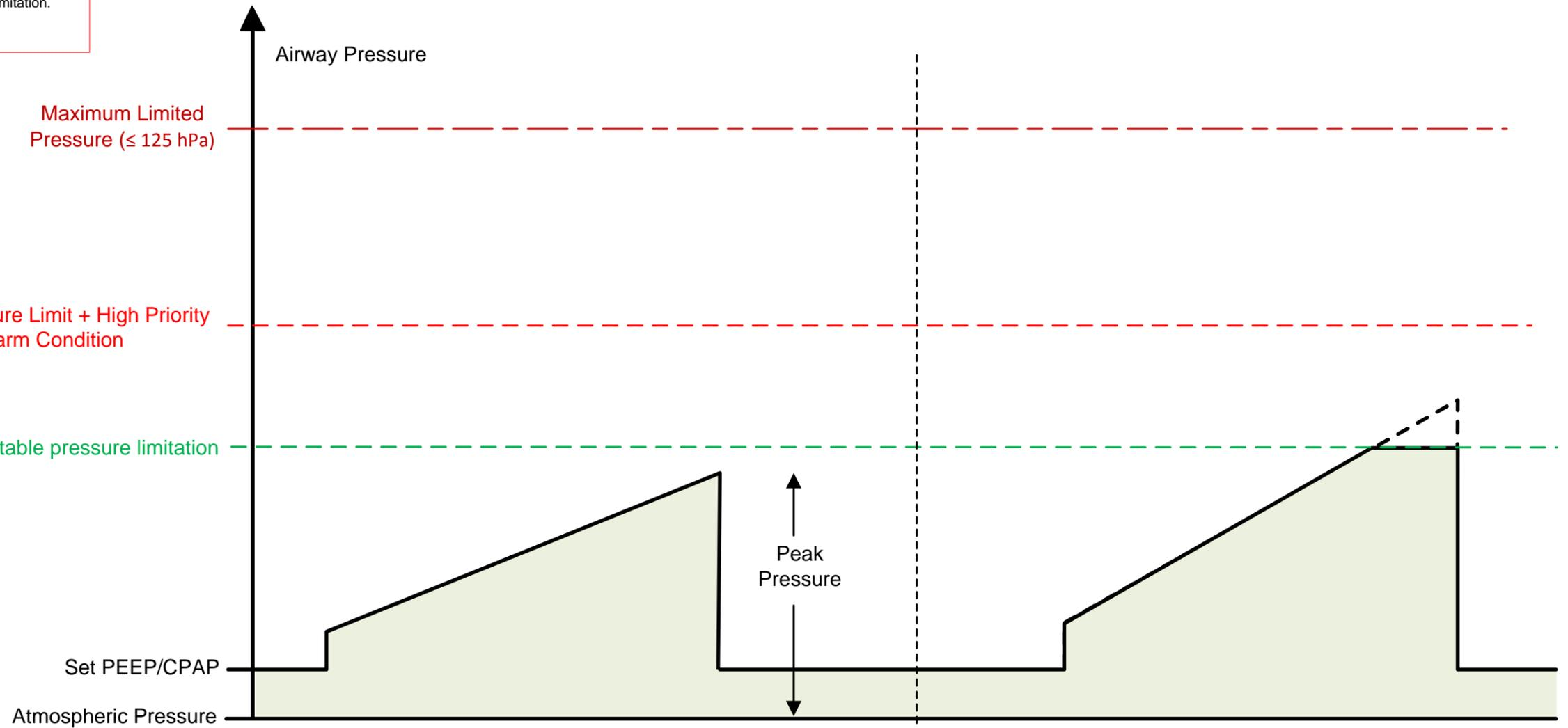
This second trace demonstrates the increase in end inspiratory pressure that may occur due to changes in the patient's lung characteristics while being ventilated with a VC breath-type. The set pressure limitation ensures that even with such changes the lung is protected from excessive pressure without creating a nuisance by generating alarms unless the consequent loss of delivered volume becomes excessive.
