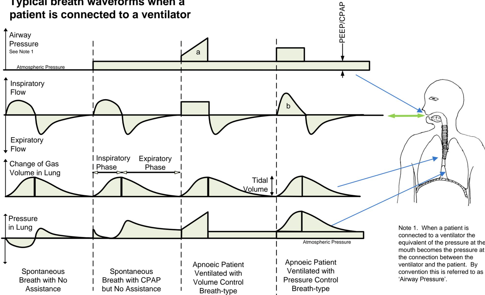
Note 1. When a patient is connected to a ventilator the equivalent of the pressure at the mouth becomes the pressure at the connection between the ventilator and the patient. By convention this is referred to as 'Airway Pressure'.
