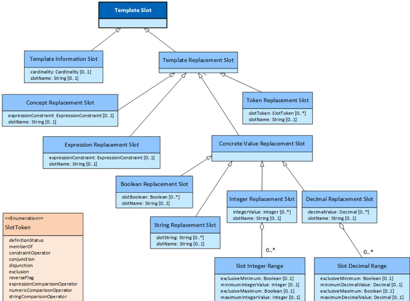
**Figure 4.1-1: UML class diagram of template syntax**
